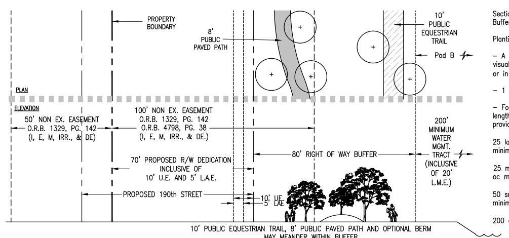
Section W - 80' Perimeter Right of Way Buffer
