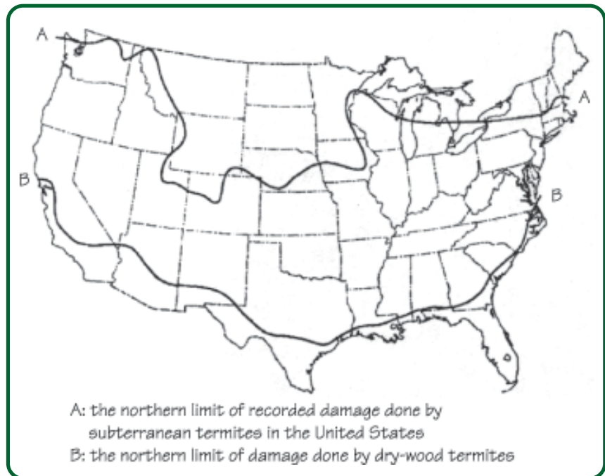
Figure 6.2 - Extent of Recorded Termite Damage
