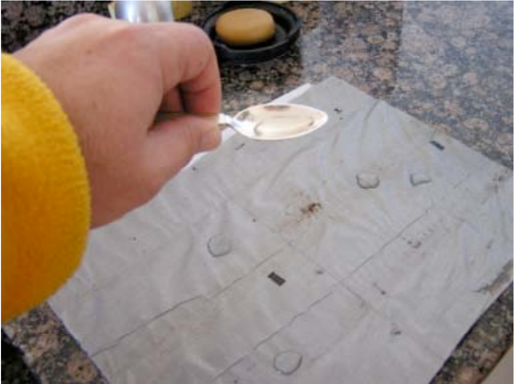
Photograph 5: Water Drop Test For Water Repellency
