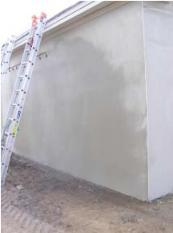
Photograph 59: Water Testing – Control Joints
