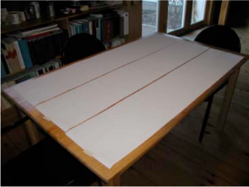
Photograph 7: Absorptive Surface For Water Drop Test
