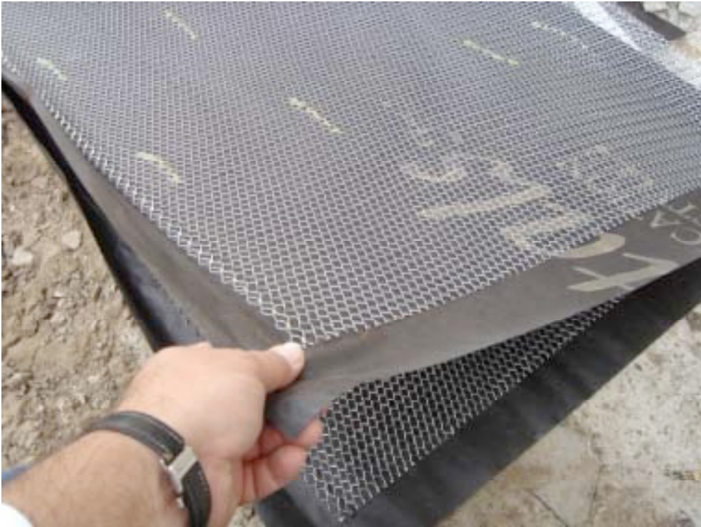
Photograph 12: Paper Backed Lath As A Bond Break
