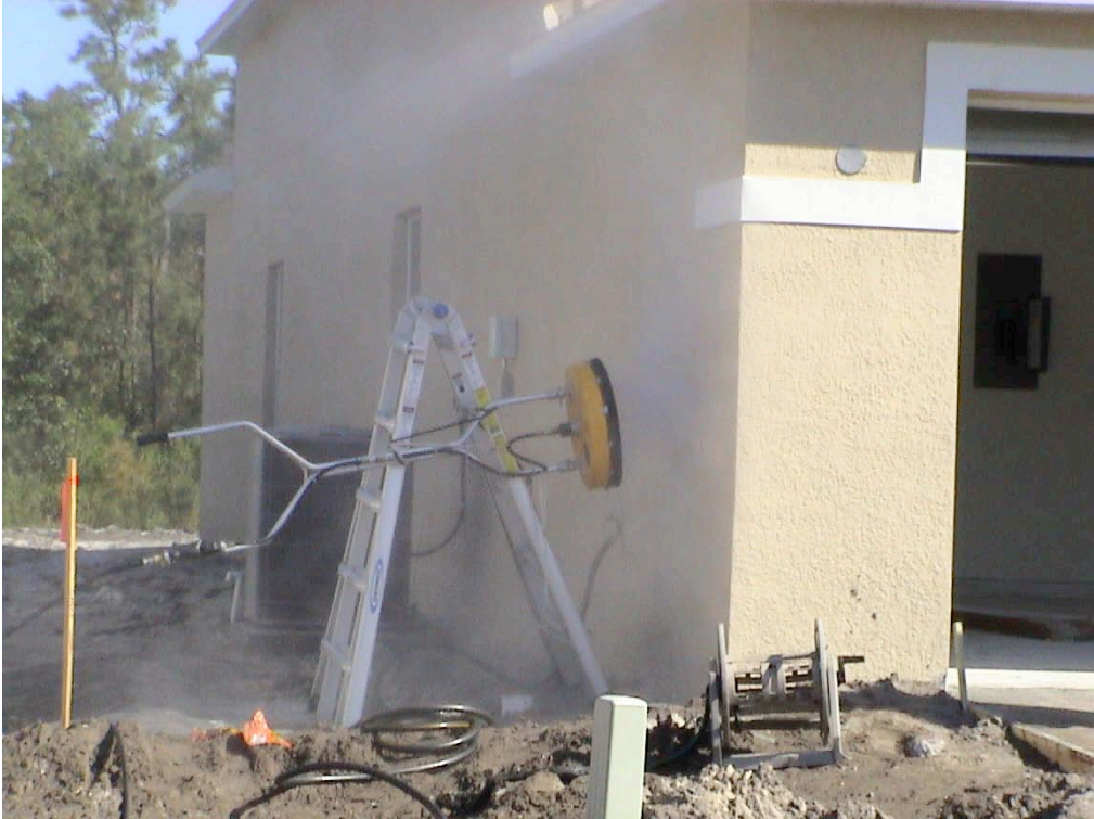
Photograph 49: Power Washer Simulating Wind Driven Rain
