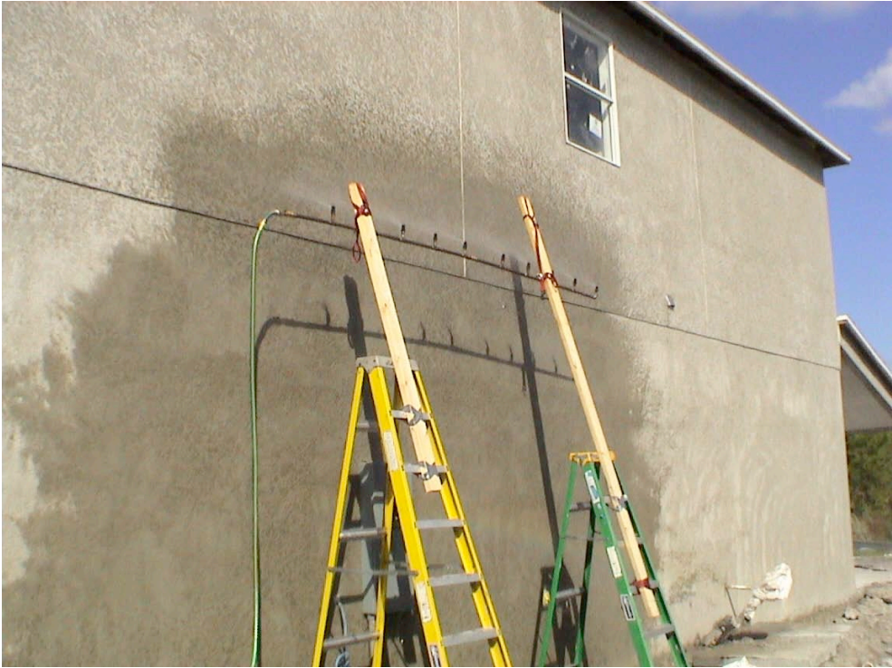
Photograph 49: Power Washer Simulating Wind Driven Rain
