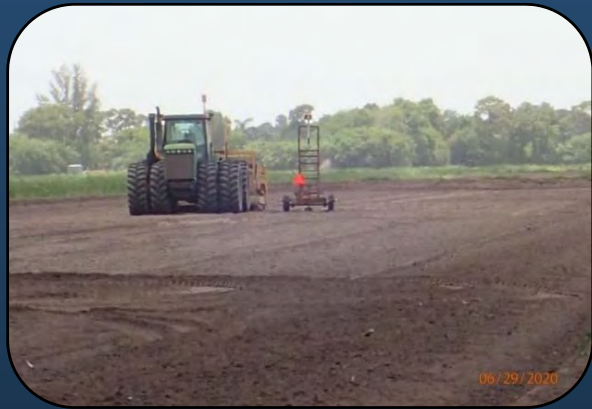
Laser leveling fields for improved subsurface irrigation
