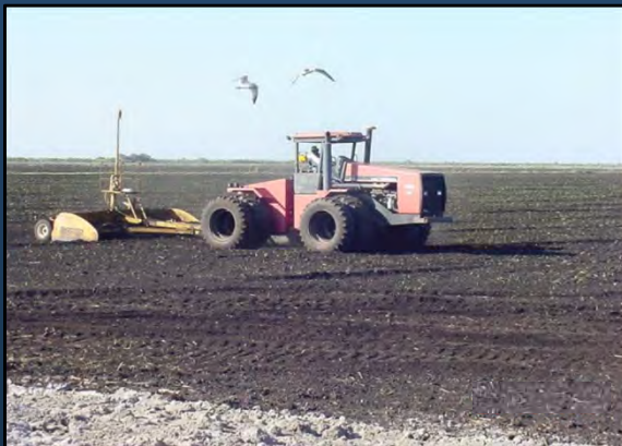
Laser leveling reduces sediment transport
