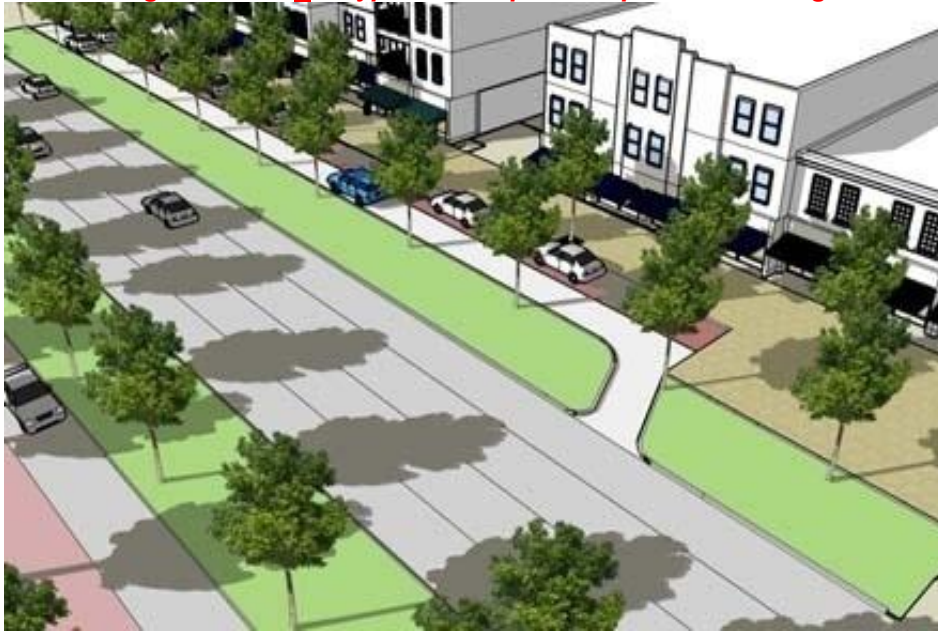
Figure 3.B.16.F – Typical Example of Slip Street Frontage
