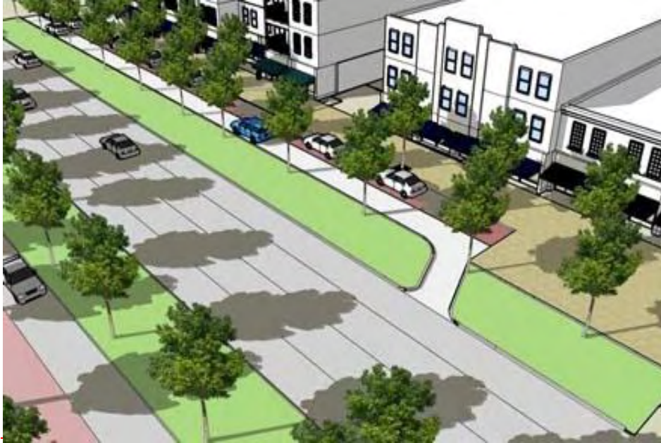
Figure 3.B.16.E – Typical Example of Slip Street Frontage
