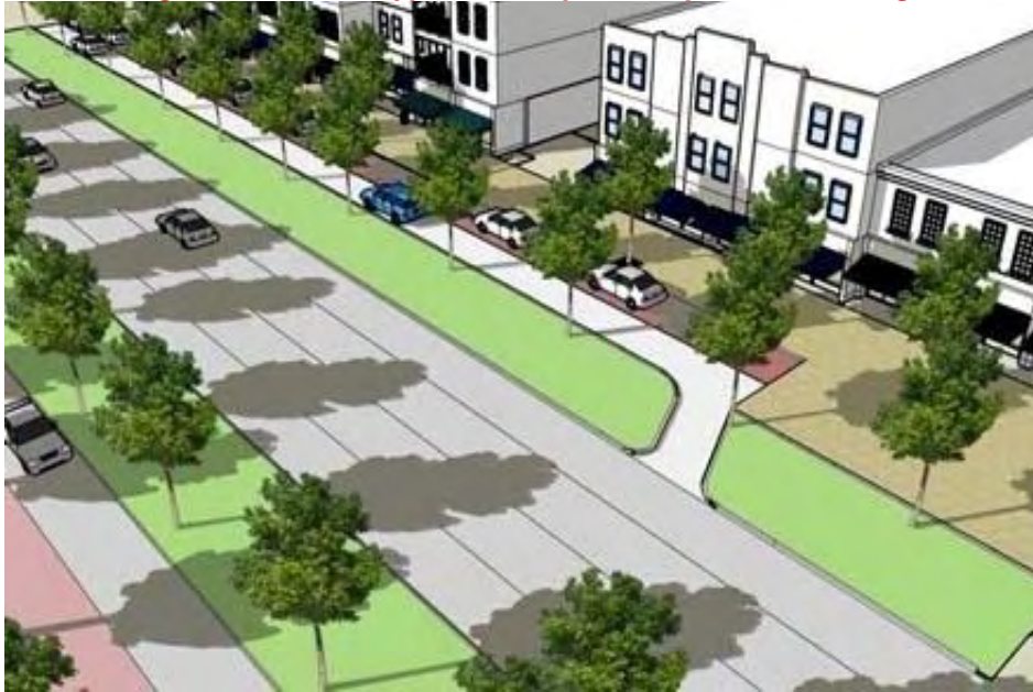
Figure 3.B.16.E – Typical Example of Slip Street Frontage
