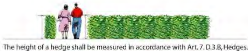
Figure 1.C.4.C - Typical Example of Measurement of Hedge Height
