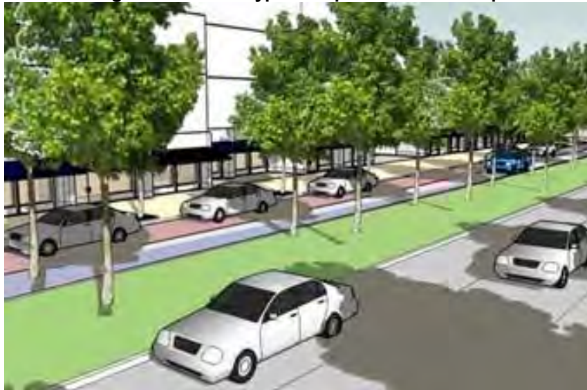
Figure 3.B.15.F - Typical Slip Street Streetscape
