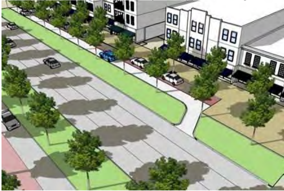
Figure 3.B.16.F - Typical Example of Slip Street Frontage
