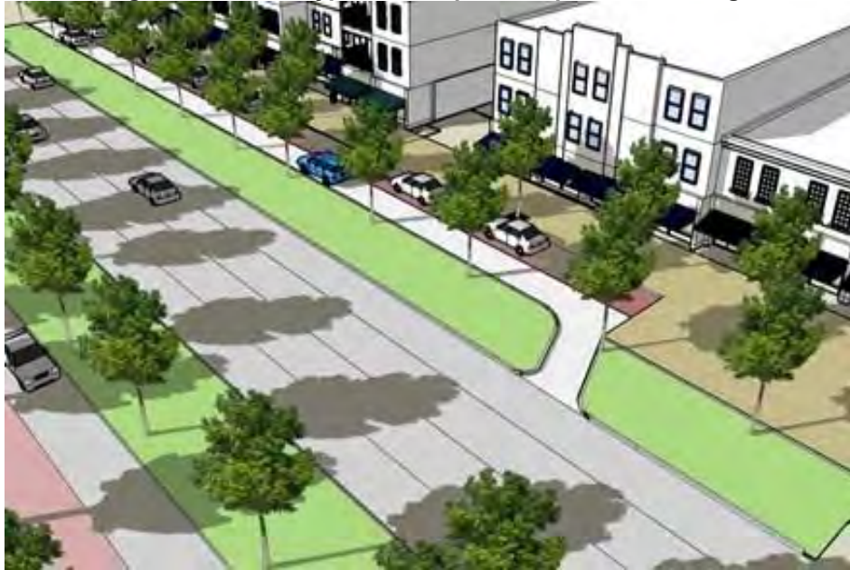
Figure 3.B.16.F - Typical Example of Slip Street Frontage
