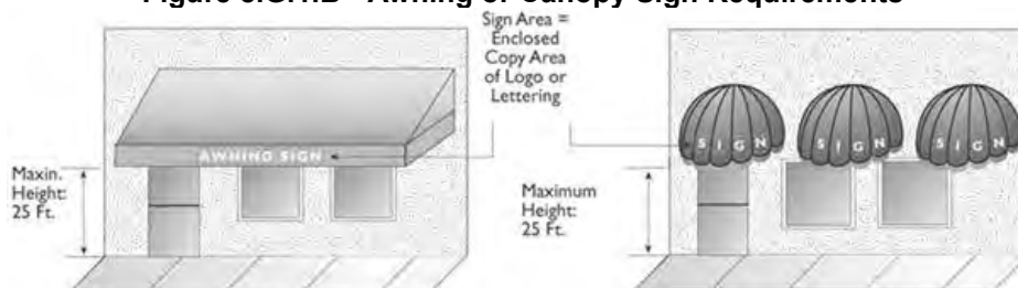
Figure 8.G.1.B - Awning or Canopy Sign Requirements
