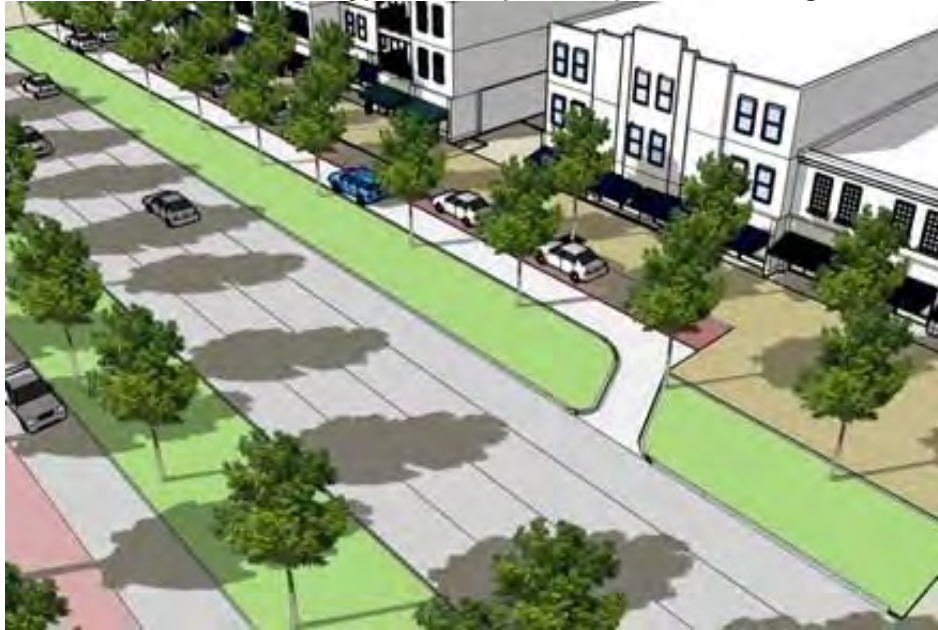
Figure 3.B.16.F - Typical Example of Slip Street Frontage
