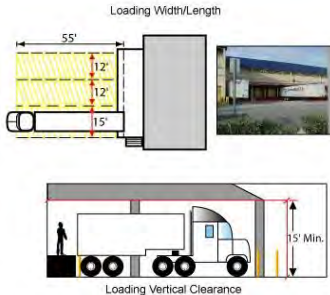
Figure 6. B.1.E - Vertical Clearance
