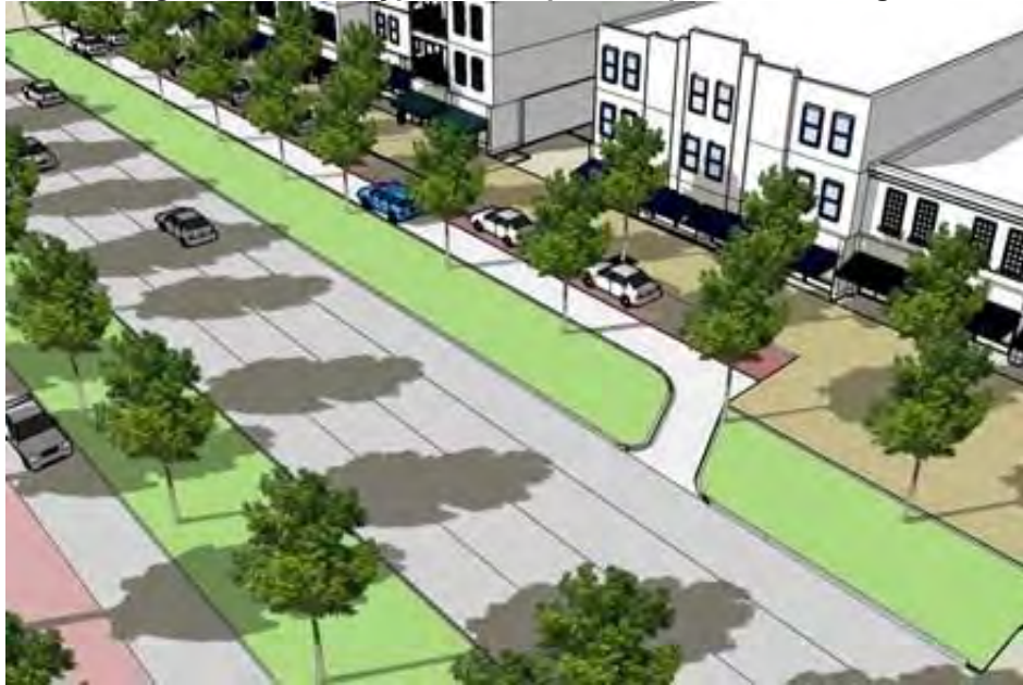
Figure 3.B.16.F - Typical Example of Slip Street Frontage
