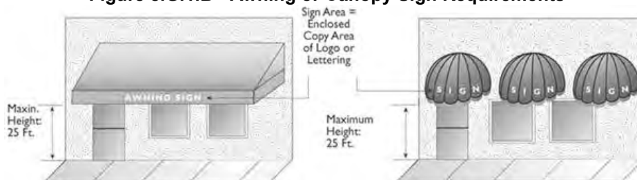
Figure 8.G.1.B - Awning or Canopy Sign Requirements
