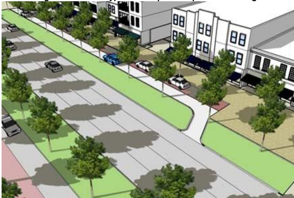
Figure 3.B.16.F - Typical Example of Slip Street Frontage
