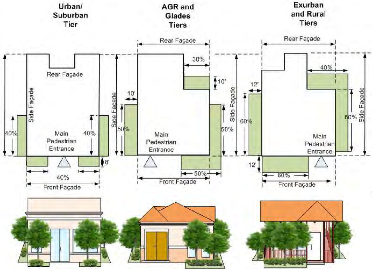
Figure 7.C.3.B – Foundation Planting Requirements
