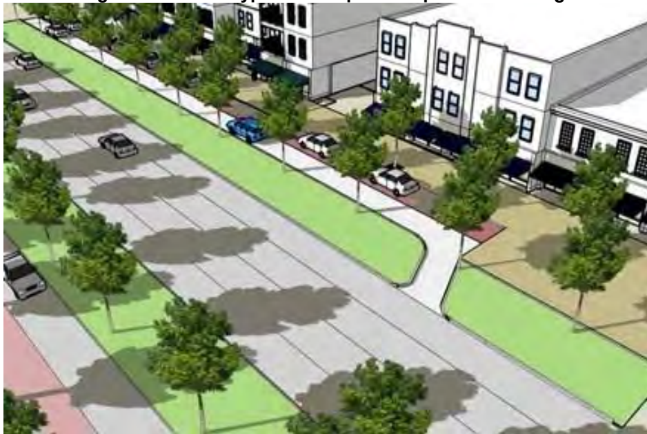
Figure 3.B.16.F - Typical Example of Slip Street Frontage
