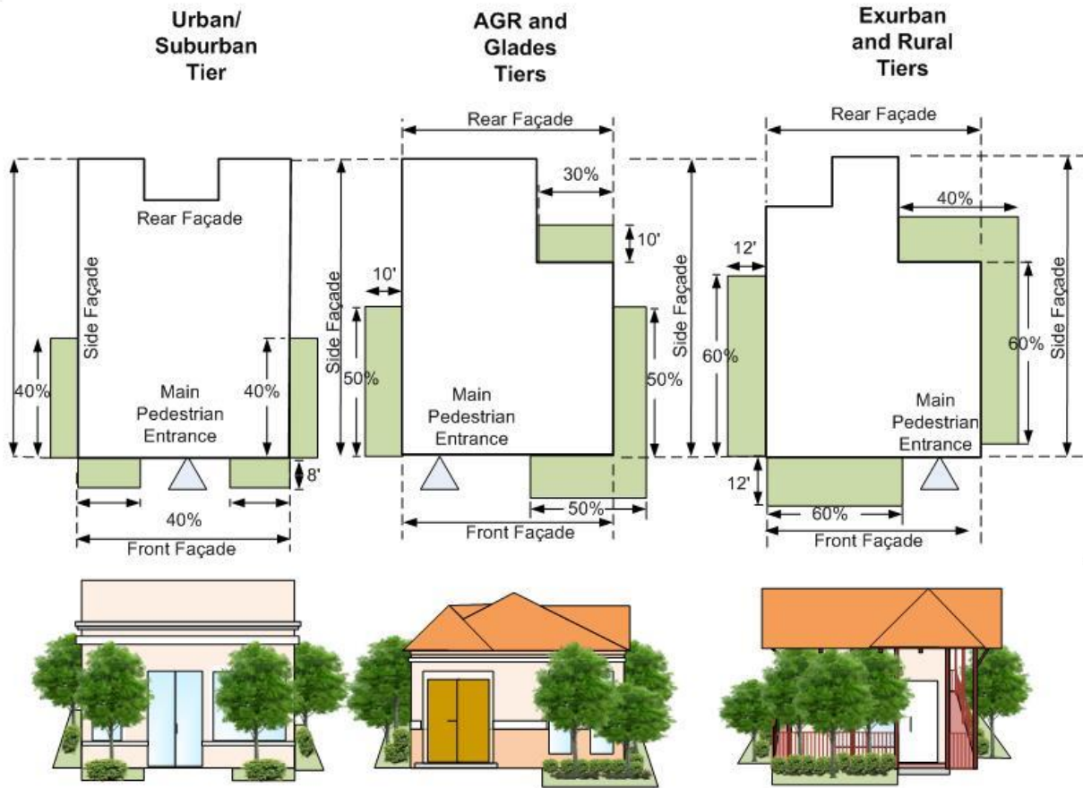
Figure 7.C.3.B – Foundation Planting Requirements
