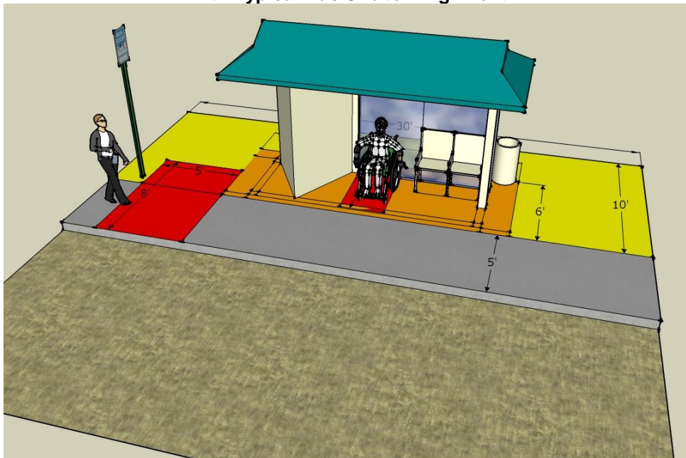
Figure 5.H.2.B – 10-foot by 30-foot Bus Stop Boarding and Alighting Area with Typical Bus Shelter Alignment
