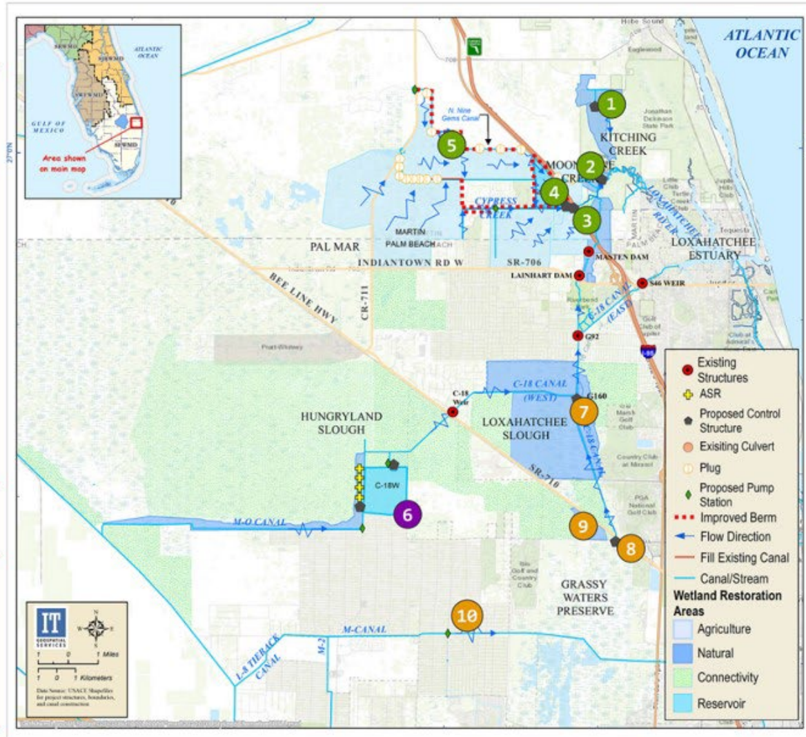
Figure 1-4. Project components and flow-ways of the Authorized Plan for the Loxahatchee River Watershed Restoration Project (From: USACE 2020).
